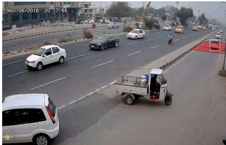
9. **No Helmet detection:** - The motor bike is becoming an increasingly utilized mode of transportation in India. Technology-related distracted motor bike and helmet use is behaviours that can impact bike safety. The proposed approach first detects bike riders from surveillance video using background subtraction and object segmentation. Then it determines whether bike-rider is using a helmet or not using visual features and binary classifier.
