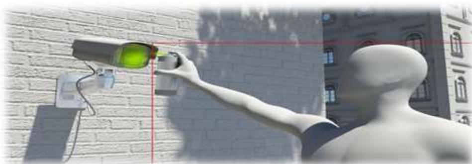
3. **Intrusion Detection:** - Video based Intrusion detection (VID) is a way of defining activity in a scene by analysing image data. It allows you to set the activity threshold and sensitivity for indoor or outdoor depending on what you want to monitor to avoid false alarms. The algorithm analyses the video frames and outputs the location of moving targets within the frame
